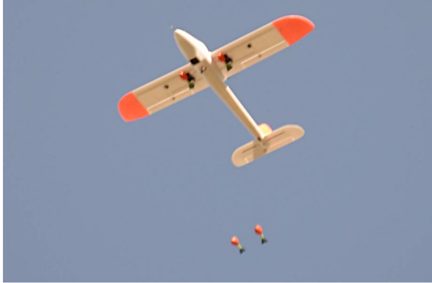
Figure 7. Autonomously controlled "ordnance" release from the Penguin UAV.
