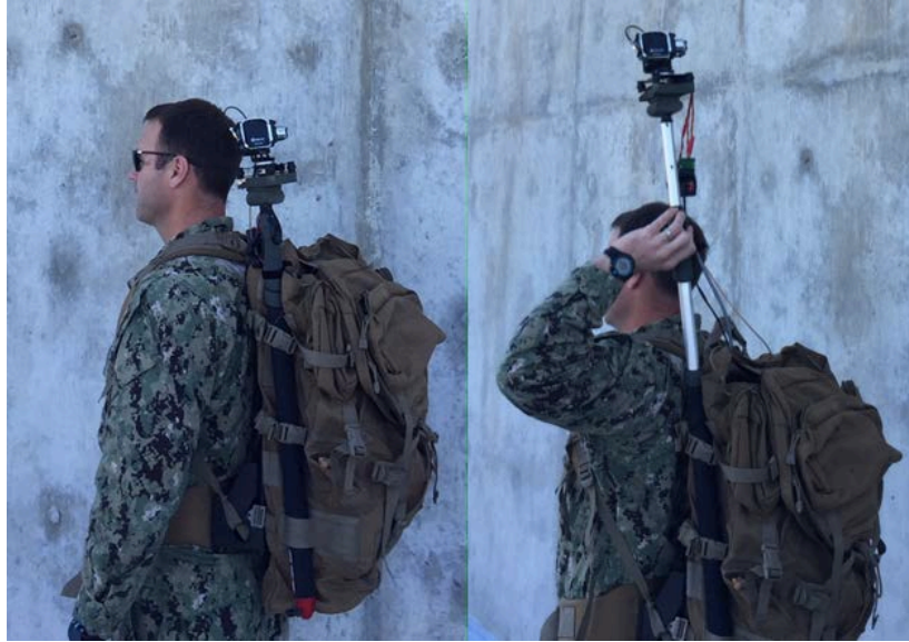
Figure 5. 3D Printed man-wearable miniature steerable directional antenna prototype.
