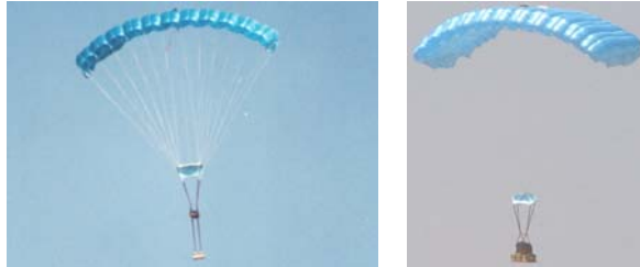
Figure 3. Generic parafoil-payload system with different ways of payload attachment.
