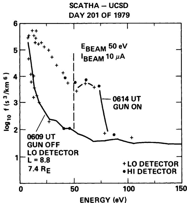
Figure 3. Electron distribution functions at 90° pitch angle, from the LO and HI detectors. Satellite is at 7.4 R<sub>E</sub> geocentric, L = 8.8, magnetic latitude 17°, 0125 MLT.
