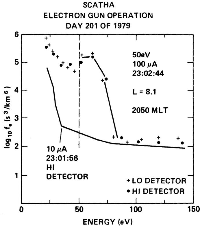
Figure 8. Electron distribution functions for 10 and 100  $\mu$ A experiments in the dusk bulge. The satellite is at 7.5  $R_E$ ,  $L = 8.1$ , magnetic latitude  $6^\circ$ , 2050 MLT.
