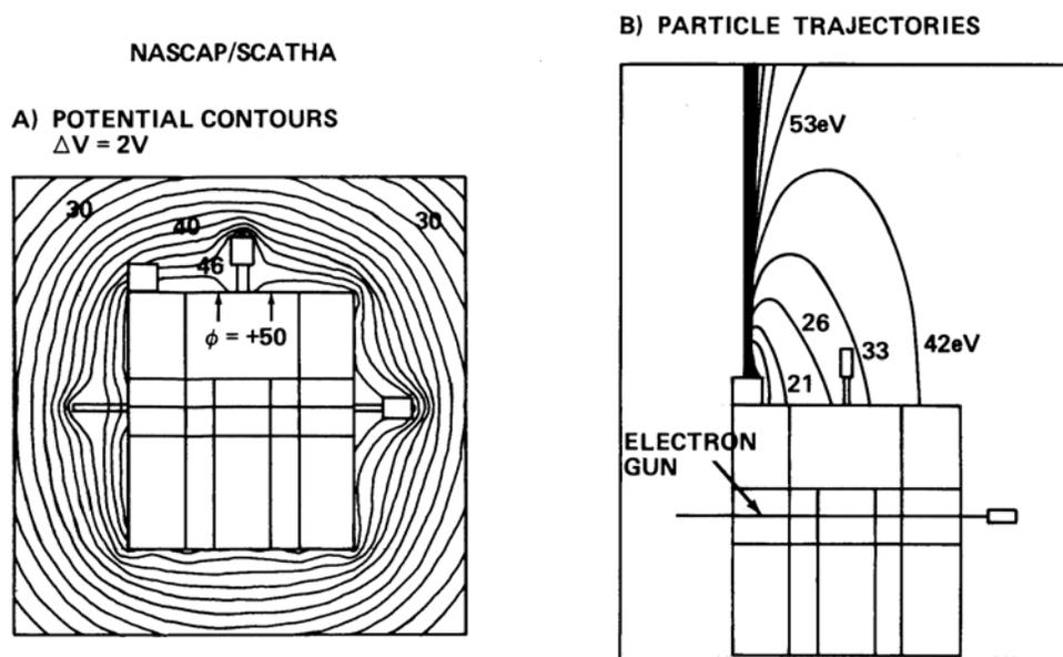
Figure 11. (a) NASCAP/SCATHA potential contours for a satellite charged to near beam energy. (b) NASCAP/SCATHA particle trajectories for electrons measured by UCSD detectors.
