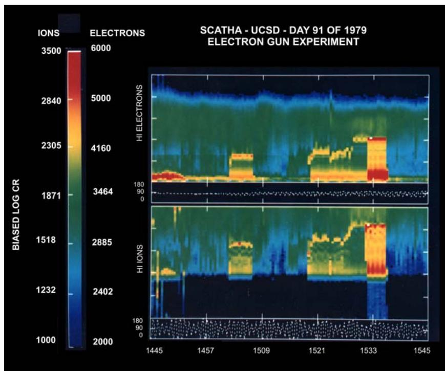
Figure 9. Energy-time spectrograms for the two UCSD electron detectors.
