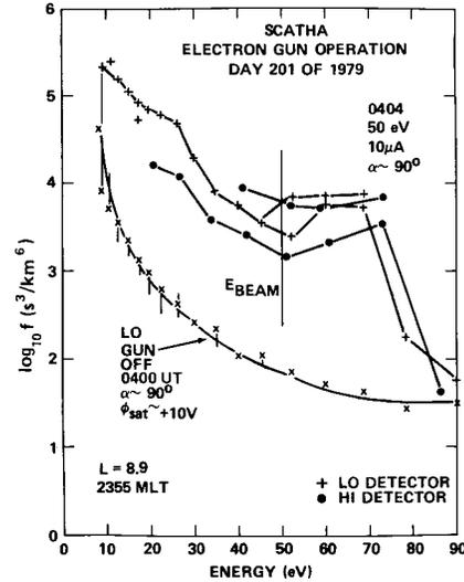
Figure 6. Electron distribution functions for zero beam current, and 10  $\mu\text{A}$  beam current.
