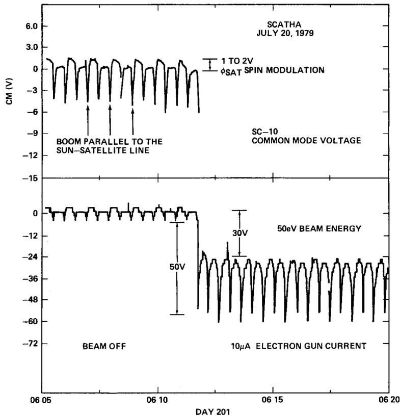
Figure 4 Common mode voltages at two ranges. The top section is from the  $\pm 15$  V channel, the bottom section from the  $\pm 300$  V channel.
