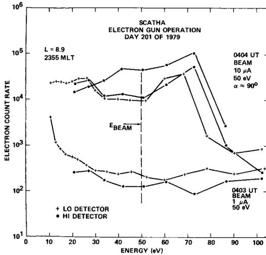
Figure 5. Electron count rate for electron gun currents of 1  $\mu\text{A}$  and 10  $\mu\text{A}$ . Satellite is at 7.7 RE geocentric,  $L = 8.9$ , magnetic latitude  $14^\circ$ , 2355 MLT.
