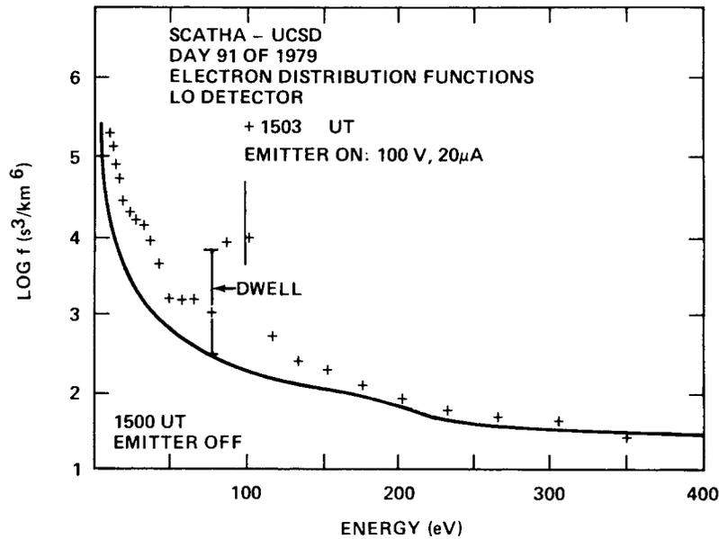
Figure 10. Electron distribution functions for 0 and 20  $\mu\text{A}$  current levels, 100 V bias on the filament electron emitter.
