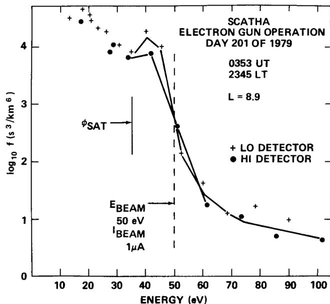
Figure 7. Electron distribution functions for 1 μA beam current in the tail lobe. Satellite is at 7.7 RE, L = 8.9, magnetic latitude 14°, 2345 MLT.
