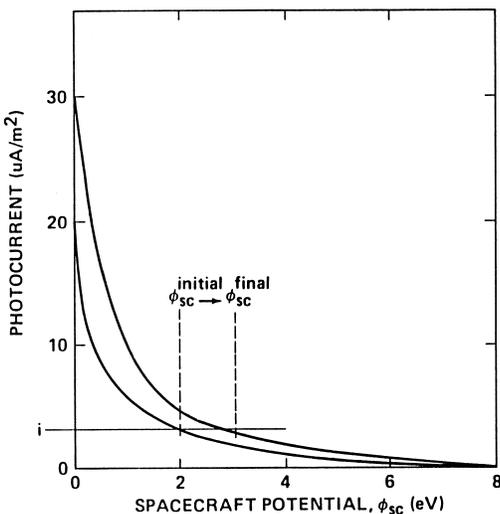
Fig. 10 A representation of the photocurrent from a surface as a function of the potential of the surface.
