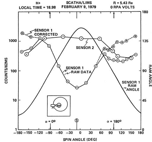
Fig. 3 A plot of H<sup>+</sup> counts per accumulation period for the LIMS.
