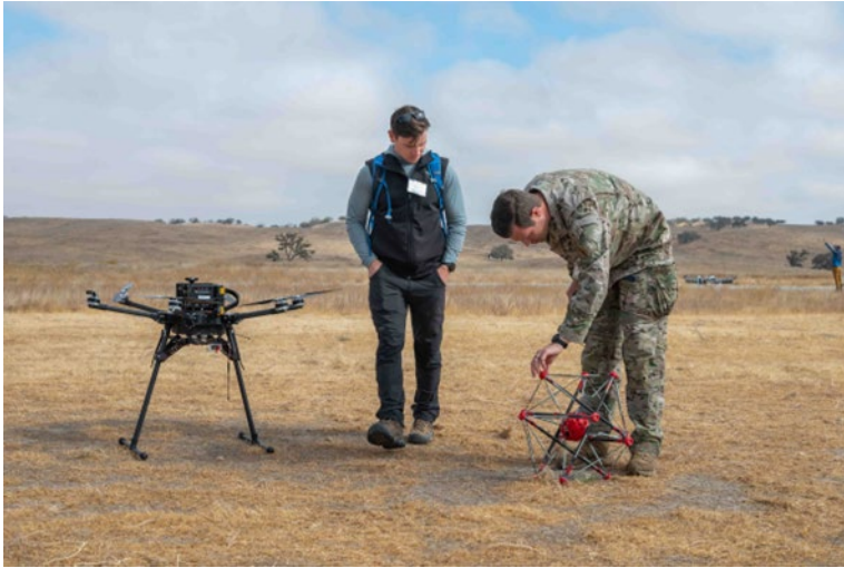
MAJ Walter Snook, NPS DA, and MSG Scott Moore, USASOC, examine Squishy Robotics' air drop capable sensor system.
