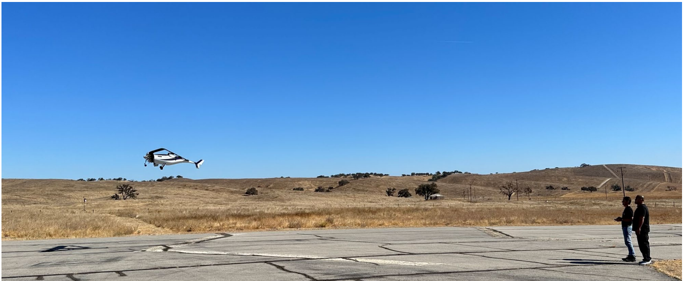
Odys Aviation’s Casper subscale research aircraft transitions from vertical takeoff to horizontal flight.
