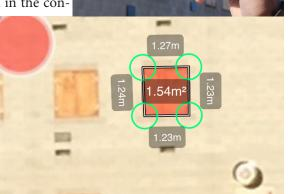
Image taken with Spike of an accurately measured window of a CACTF building at a 100m range.
