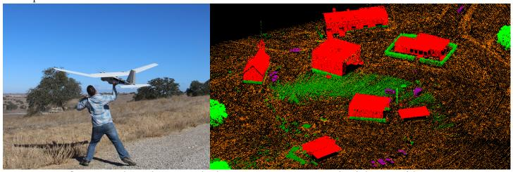
Aero Vironment flew a new, advanced LiDAR payload in its Puma UAV generating detailed images of the CACTF site.
