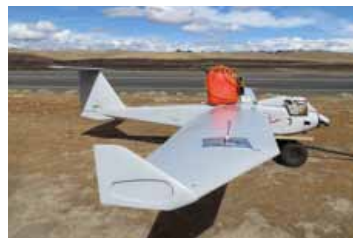
Fig 5 ADS-B antenna on Arcturus T20 UAV
