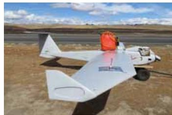
Fig 5 ADS-B antenna on Arcturus T20 UAV
