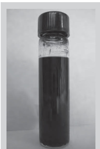
Figure 6. Nano-reinforced matrix resin consisting of a very stable colloidal suspension of SWNTs in Derakane 510 vinyl ester resin with controlled viscosity.
