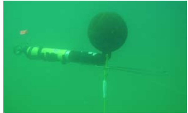
Ranger AUV attaches to mine-like object, using feature-based algorithms to localize and navigate with limited sensors.
