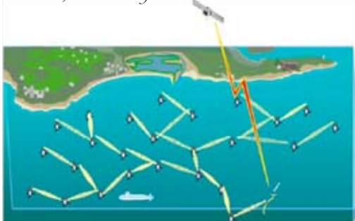
Seaweb underwater network, showing acoustic links between buoys and submersibles, possible satellite links
