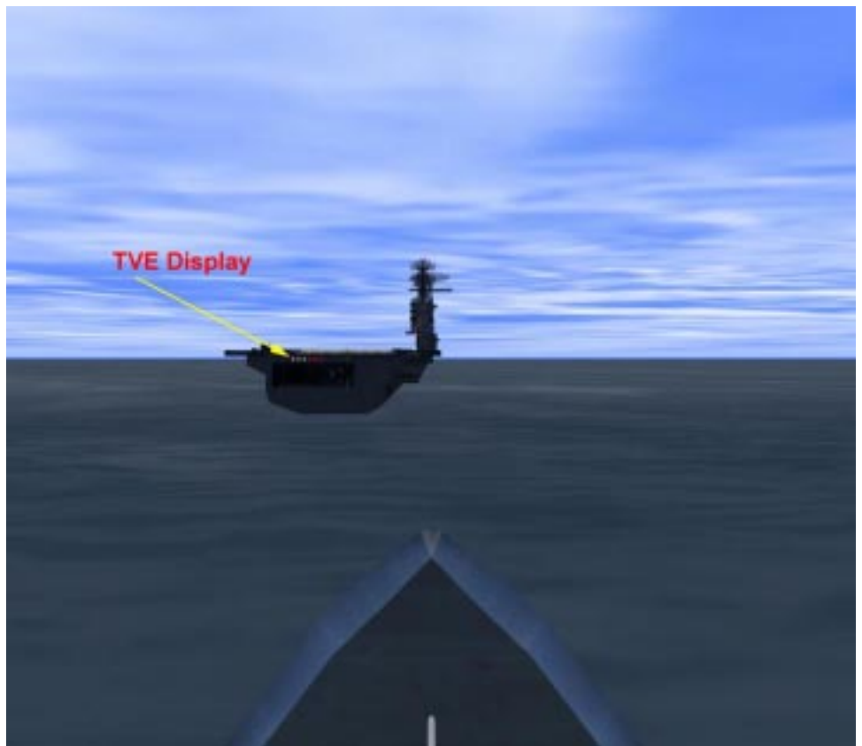
Figure 1. The Tactical Vectoring Equipment (TVE) shipboard navigation display resulted from the thesis work of LCDR Evanoff to design and analyze a shipboard visual navigation aid for vessels in formation. The TVE display contains a horizontal line of its bicolor (red and white) lights spaced approximately six feet apart on the stern of the carrier.
