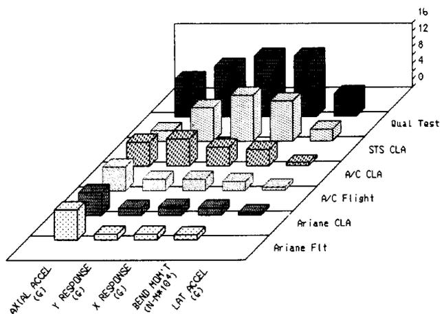
Figure 2. Peak Acceleration Comparison
