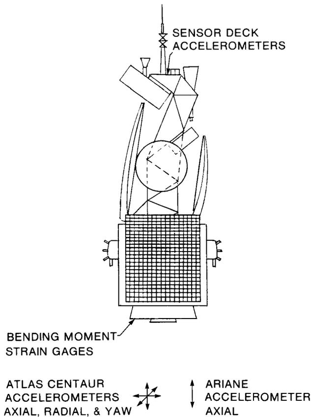
Figure 1. INTELSAT V Instrumentation Location
