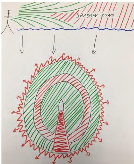
Figure 30. Traditional sensor display where sensor coverage is green and shadow zones in red illustrating gaps in coverage hidden by “circle of coverage” displays, side-view (top) and overhead view (bottom).
