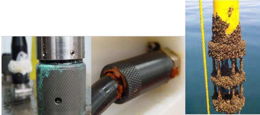
Figure 12. Corrosion<sup>5</sup> (left) and biofouling<sup>6</sup> (right) are common causes of sensor failure.
