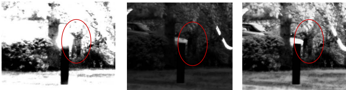
Figure 38. The UV image of the camouflage uniform set-up presented in its respective red (left), green (center) and blue (left) channels. Notice the best contrast is in the blue channel.
