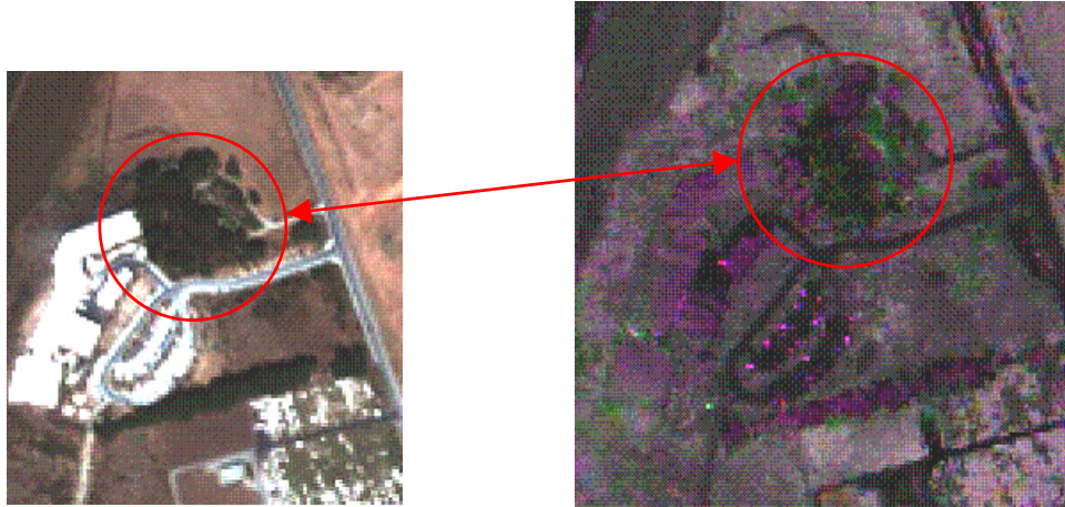
Figure 36. QuickBird image of Monterey Cypress and Eucalyptus Trees (left) LIDAR Intensity image of corresponding Quickbird Image; Eucalyptus Trees appear Dark, Cypress Trees Appear Purple; Band 1 is Mapped to Red, Band 2 is Mapped to Green, and Band 3 is Mapped to Blue (right)
