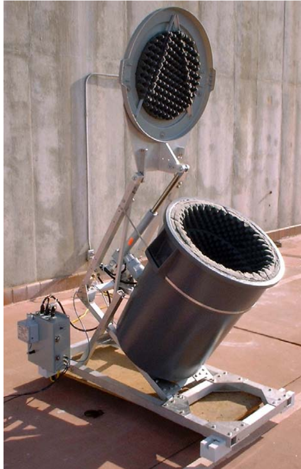
Figure 2. Acoustic sounder designed and built by Professor Donald Walters and Jay Adeff at the Naval Postgraduate School.
