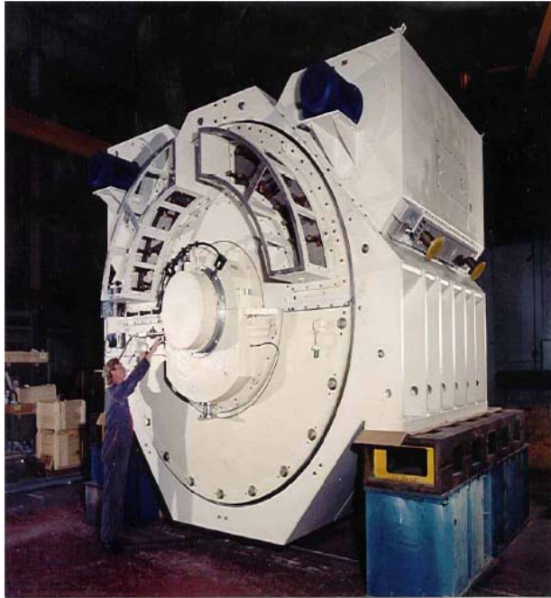
Figure 197. Alstom 19MW Advanced Induction Motor 12
