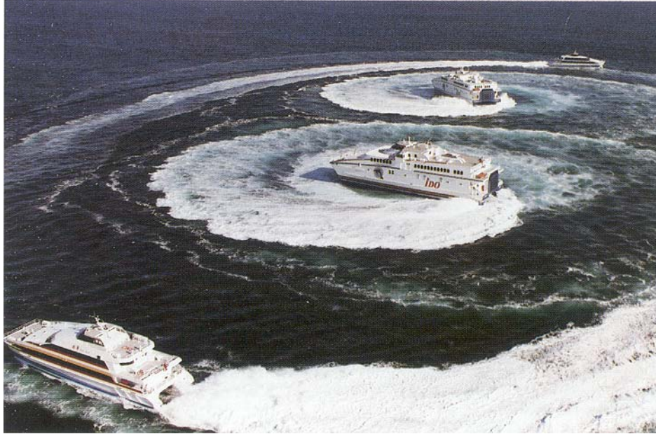
Figure 8 Maneuvering waterjet equipped vessels with Steering and Reversing Systems from Reference [5].
