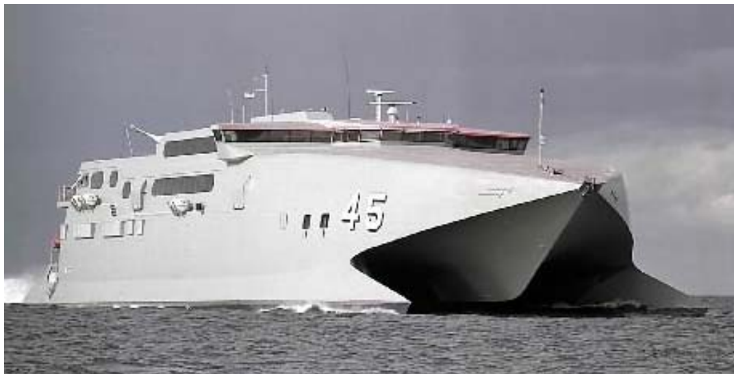
Figure 11 Typical Wave Piercing Bow from Reference [7]
