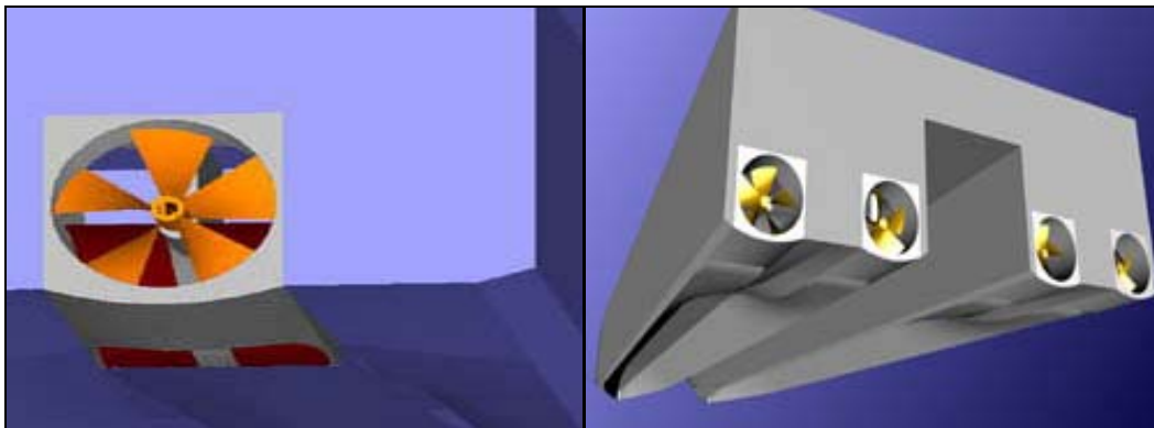
Figure 65 Typical Hydro-Air Drive Install (from Ref[48]).
