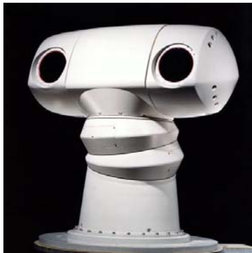
Figure 84 Notional IRST system (from [23])
