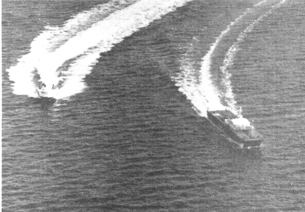
Figure 9 High Length/Beam Ratio SES Wake Comparison to Monohull from Reference [6].
