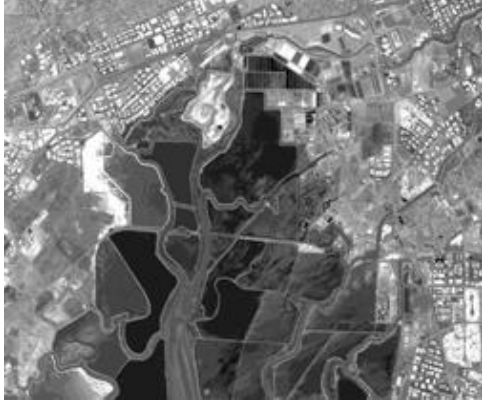
Figure 2c: Haralick Method Quantization image for the simulated MSI image. The 4 simulated MSI bands were summed to create a panchromatic image band.
