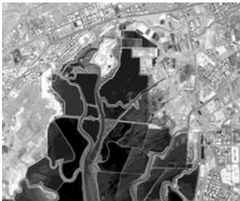
Figure 2a: Haralick Method Quantization image created for the HSI image. All 224 HSI bands were summed to simulate a panchromatic image.
