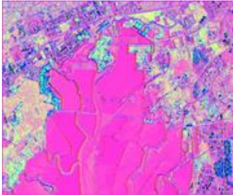
Figure 10a: RGB image of Principal Components 1-3; Haralick Method Textures from HSI image cube.
