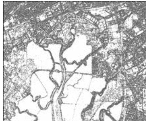
Figure 9d: Spectral Texture Method Mean texture feature for the simulated MSI image cube.
